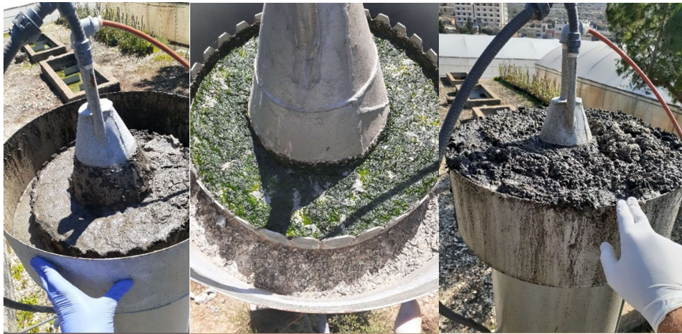
Photo 4.4: several troubleshooting photos show huge foaming layer was formed, and overflowed from the top of the reactor causing an outlet tube blockage and a big bio solids washout. (Date:17.11.2019)
