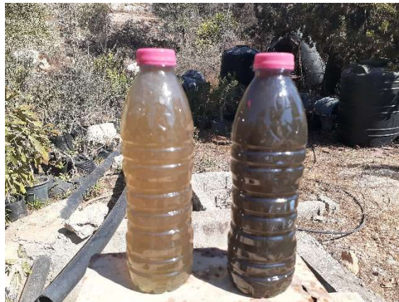
Photo 4.1: influent Vs Effluent visual results, 3 months' operation. (Date: 30.09.2019)
