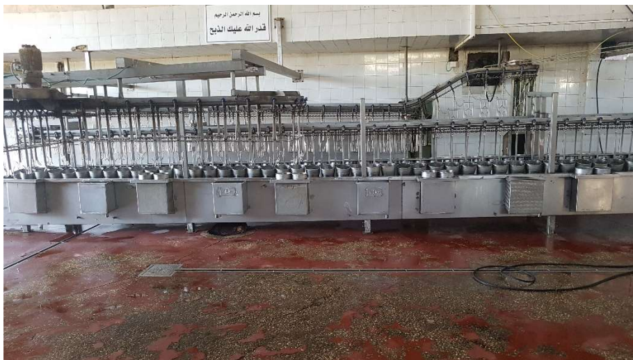
Photo A-3: Poultry Slaughterhouse blood collection system
